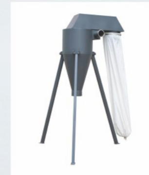
旋风分离回收装置 Cyclone Separation and Recovery Unit
